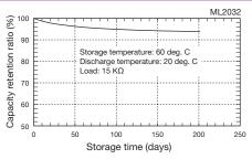
(when accelerating 20 days at 60 deg. C equivalent to 1 year at 20 deg. C)
