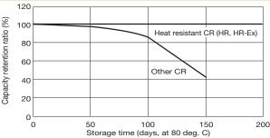
Very little deterioration in capacity due to high storage temperature of 80 deg. C, compared to other CR batteries.
