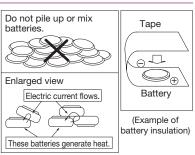
so make sure to cover the (+) and (-) terminals with friction tape or some other insulator before disposal.
