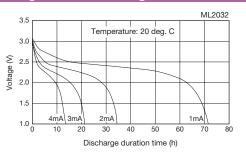
Maxell). And since organic electrolyte is used, the battery has superior leakage resistance (shipped fully charged).
