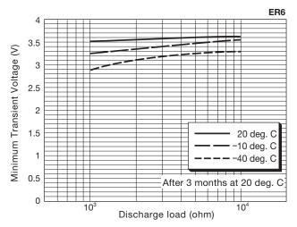
The figure above shows minimum transient voltage using a fresh battery.
