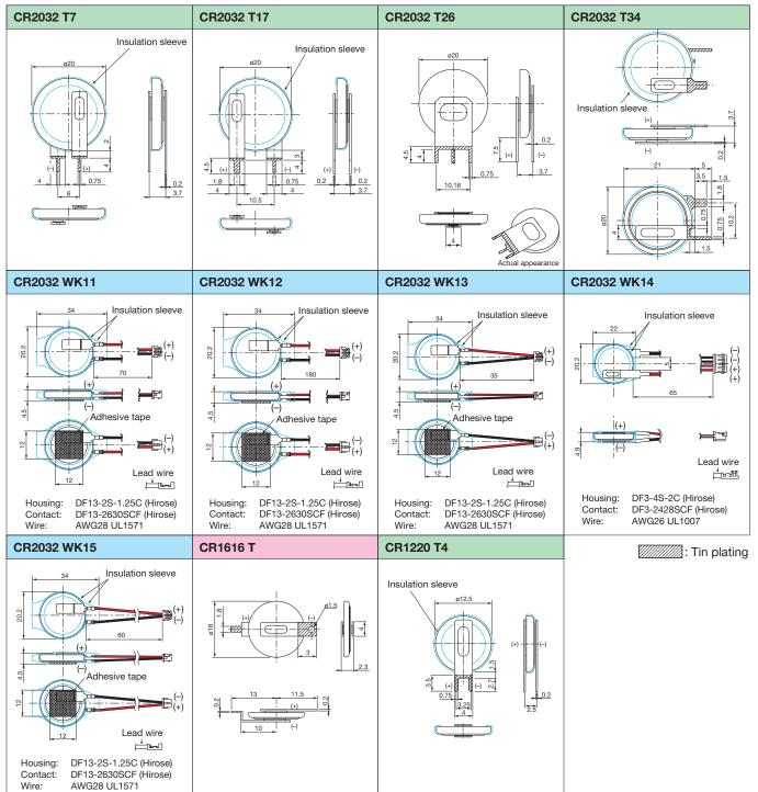
: Horizontal & Through hole Type : Horizontal & Surface mounting Type : Vertical & Through hole Type : Wire connector Type
