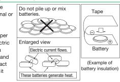
overheating, or explosion, so make sure to cover the (+) and (-) terminals with friction tape or some other insulator before disposal.
