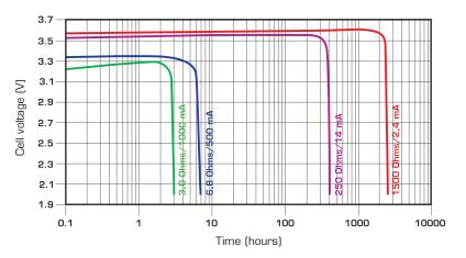
Typical discharge profiles at + 20°C
