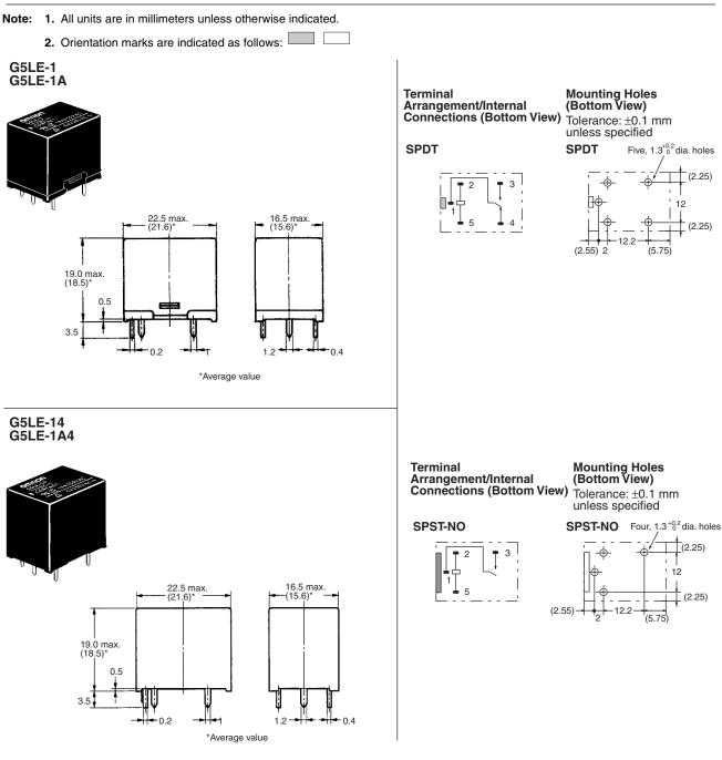
ALL DIMENSIONS SHOWN ARE IN MILLIMETERS. To convert millimeters into inches, multiply by 0.03937. To convert grams into ounces, multiply by 0.03527.
