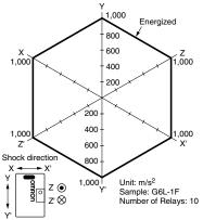
Conditions: Shock is applied in  $\pm X$ ,  $\pm Y$ , and  $\pm Z$ directions three times each with and without energizing the Relays to check the number of contact malfunctions
