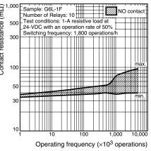
The contact resistance data are periodically measured reference values and are not values from each monitoring operation. Contact resistance values will vary according to the switching frequency and operating environment, so be sure to check operation under the actual operating conditions before use. 2.
