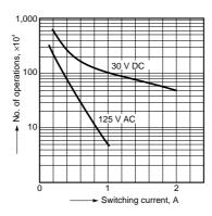
3. Contact reliability for AC loads Tested sample: DS2E-M-DC24V 10 pcs. Operating speed: 20 cpm.
