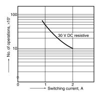
4. Mechanical life Tested sample: TK1-12V, 8 pcs. Switching frequency: 30 Hz
